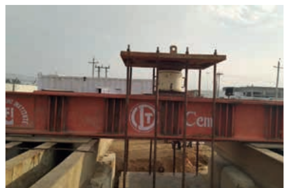
Pull out (Tension) Loading Test 680mm dia CFA piles, 11.5m long
