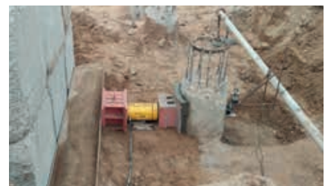
Lateral Loading Test - DFI
