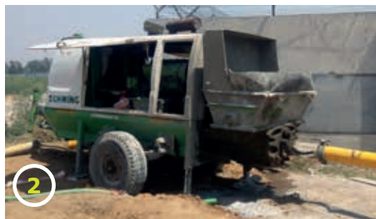
1) RMC truck and concrete, 2) grout / concrete pumping unit, 3) Automated Monitoring Unit installed within rig panel 4) grout / concrete hose, 5) Piling with hydraulic rotary rig mounted continuous flight auger and long boom crane
