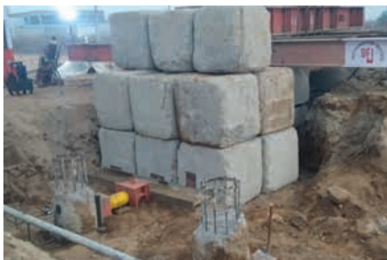
Lateral Loading Test 680mm dia CFA piles, 11.5m long
