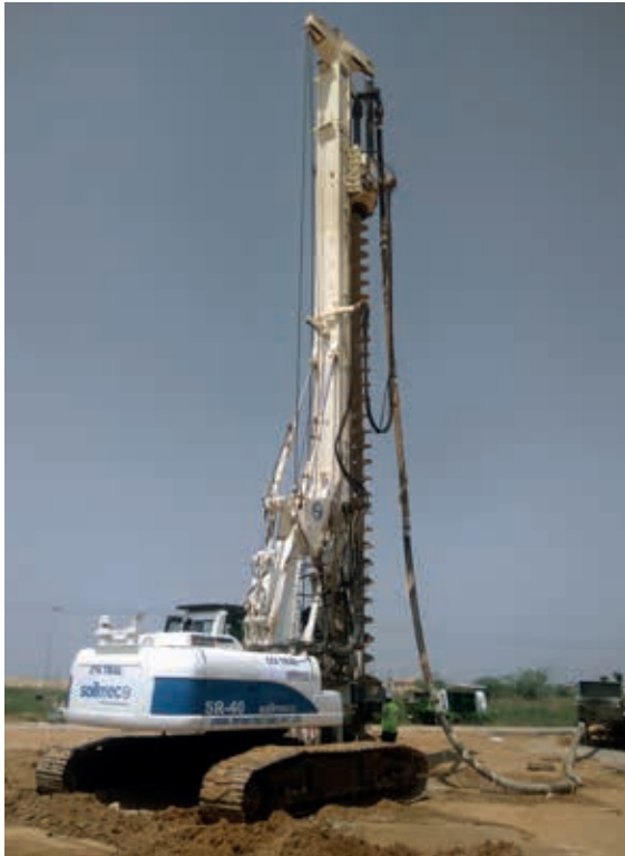
Conventional hydraulic rotary rig modified to house continuous flight auger
