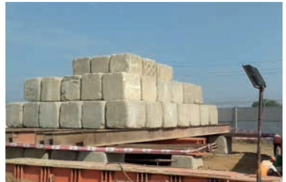
Vertical Compression 680mm dia CFA piles, 11.5m long
